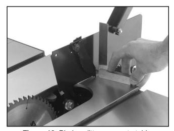
Figure 18. Blade splitter square to table.
